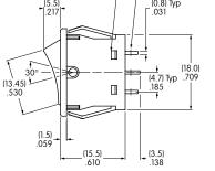
The .043" x .079" terminal hole accommodates 1 solid 18-gauge wire or 2 solid or stranded 20-gauge wires.
